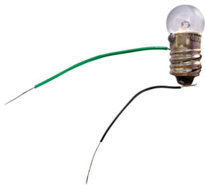
Fig.12.4 Bulb connected to two wires
