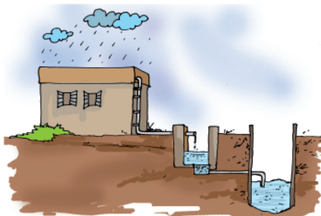
Fig. 14.13 Rooftop rainwater harvesting
