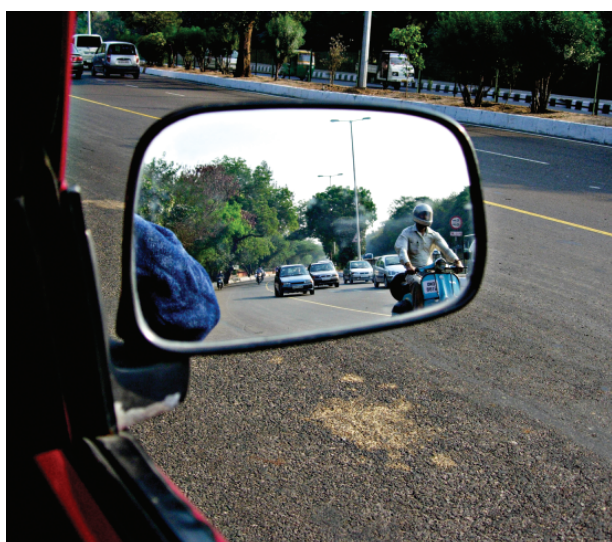
Fig. 15.20 Convex mirror as side view mirror
