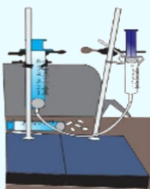
Fig10.1.13: Application of Pascal's Law- Interconnected syringes
