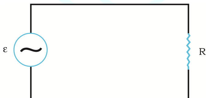
Fig. 7.1.6 Alternating current through a resistor
