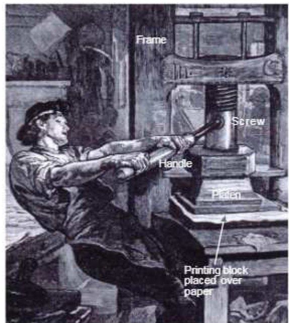
Fig. 6 – Gutenberg Printing Press.
