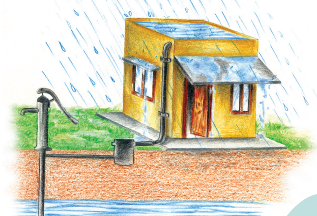
(a) Recharge through Hand Pump
