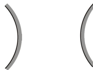
(a) Concave mirror (b) Convex mirror
