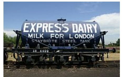
Preserved Express Dairies three-axle Milk Tank Wagon at the Didcot Railway Centre, based on an SR chassis
