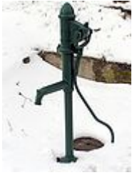
Hand-operated, reciprocating, positive displacement, water pump in Košice-Ťahanovce, Slovakia (walking beam pump).
