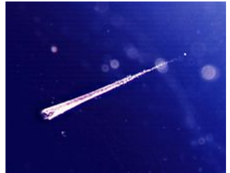
Meteoroid embedded in aerogel; the meteoroid is 10 \mu\text{m} in diameter and its track is 1.5 mm long
