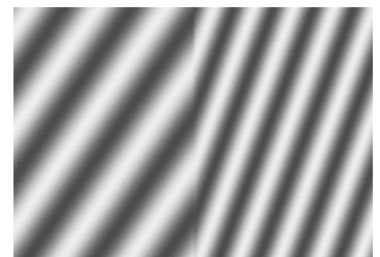
Sinusoidal traveling plane wave entering a region of lower wave velocity at an angle, illustrating the decrease in wavelength and change of direction (refraction) that results.
