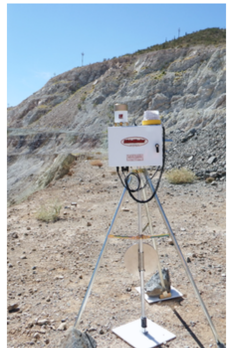
A Wireline extensometer monitoring slope displacement and transmitting data remotely via radio or Wi-Fi. In situ or strategically deployed extensometers may be used to provide early warning of a potential landslide. [20]
