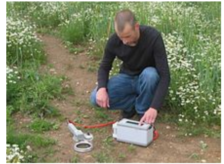
Measuring soil respiration in the field using an SRS2000 system.
