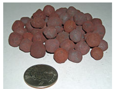
Processed taconite pellets with reddish surface oxidation as used in the steelmaking industry with a US Quarter (diameter: 24 mm (0.96 in)) shown for scale.
