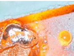
Copper just above its melting point keeps its pink luster color when enough light outshines the orange incandescence color
