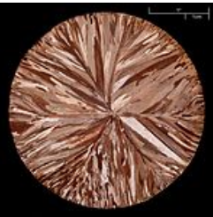
A copper disc (99.95% pure) made by continuous casting etched to reveal crystallites
