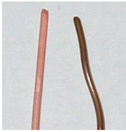
Unoxidized copper wire (left) and oxidized copper wire (right)
