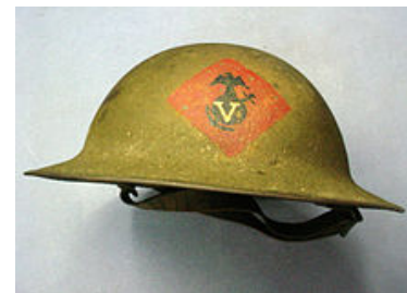
U.S. M1917 combat helmet, a variant of Brodie helmet, made from Hadfield steel manganese alloy
