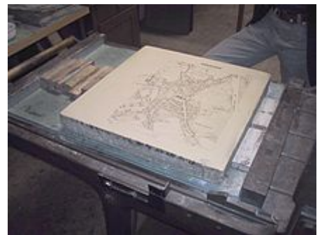
A limestone plate with a negative map of Moosburg in Bavaria is prepared for a lithography print.
