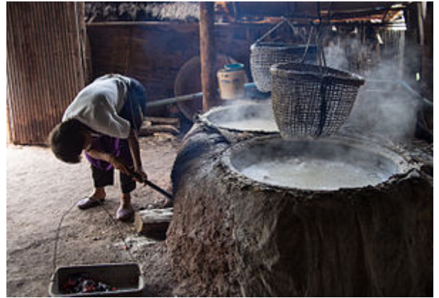
Brine from salt wells is boiled to produce salt at Bo Kluea, Nan Province, Thailand
