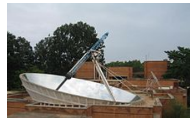
Parabolic dish produces steam for cooking, in Auroville, India
