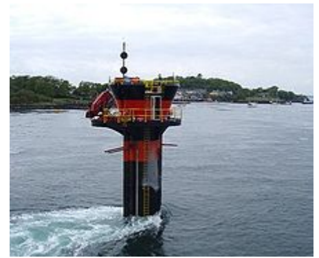
The world's first commercial-scale and grid-connected tidal stream generator – SeaGen – in Strangford Lough. [9] The strong wake shows the power in the tidal current
