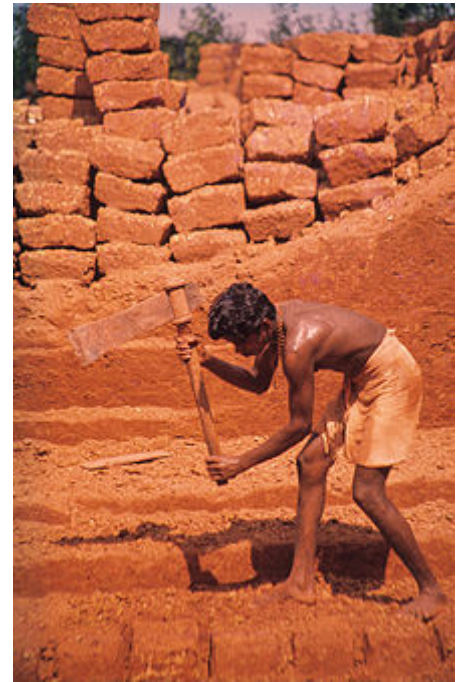
Cutting laterite bricks in Angadipuram, India
