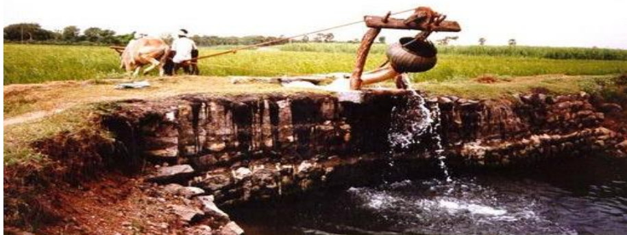
Ancient Method of Water Lifting (kamalai erram) from Well
