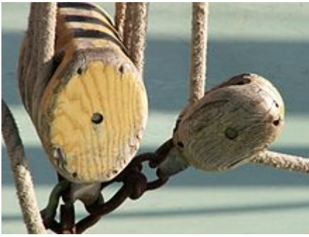
A pulley block for rigging on a sailing ship. By 1808, annual production in Portsmouth reached 130,000 blocks.
