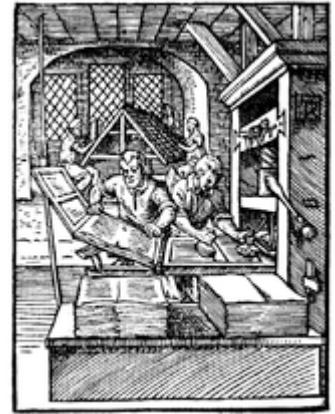
This woodcut from 1568 shows the left printer removing a page from the press while the one at right inks the text-blocks. Such a duo could reach 14,000 hand movements per working day, printing around 3,600 pages in the process. [3]
