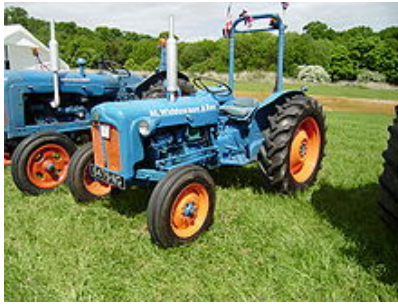
Rollover protection bar on a mid-20th century Fordson tractor
