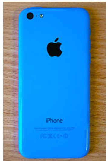
iPhone 5c, a smartphone with a polycarbonate unibody shell
