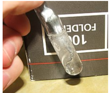
Zinc, a base metal, reacting with an acid
