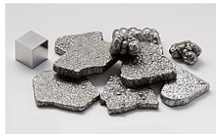
Pure (99.97%+) iron chips, electrolytically refined accompanied by a high purity (99.9999% = 6N) 1 cm 3 cube
