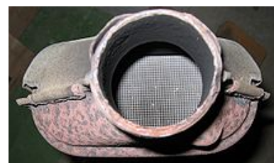
Solid heterogeneous catalysts are plated on meshes in ceramic catalytic converters in order to maximize their surface area. This exhaust converter is from a Peugeot 106 S2 1100.
